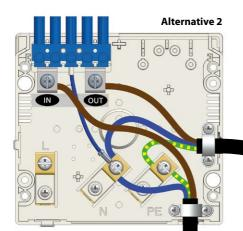
Stove Guard's maximum supply current allowed is 32A and the appropriate diversity factor is 100%. The diversity factor applies to Stove Guard installations with parallel connected relays. Type 1, or equivalent circuit breaker (MCB) shall be used for protecting the Stove Guard supply. The circuit breaker shall have capability of interrupting the supply current within 100 ms at 4 x load.
