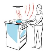
The Heat Sensor may start making short "beeps" every five seconds while it is being used ("pre-alarm").
