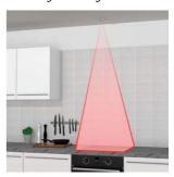
For ceiling installations, the supplied IR lens extension must also be fitted. See page 10.
