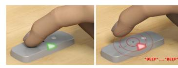
**Note:** When selecting the correct sensitivity level it is important the process is not rushed. Ensure the sensor button is pressed firmly down each time, holding for a period of 1 second before releasing.
